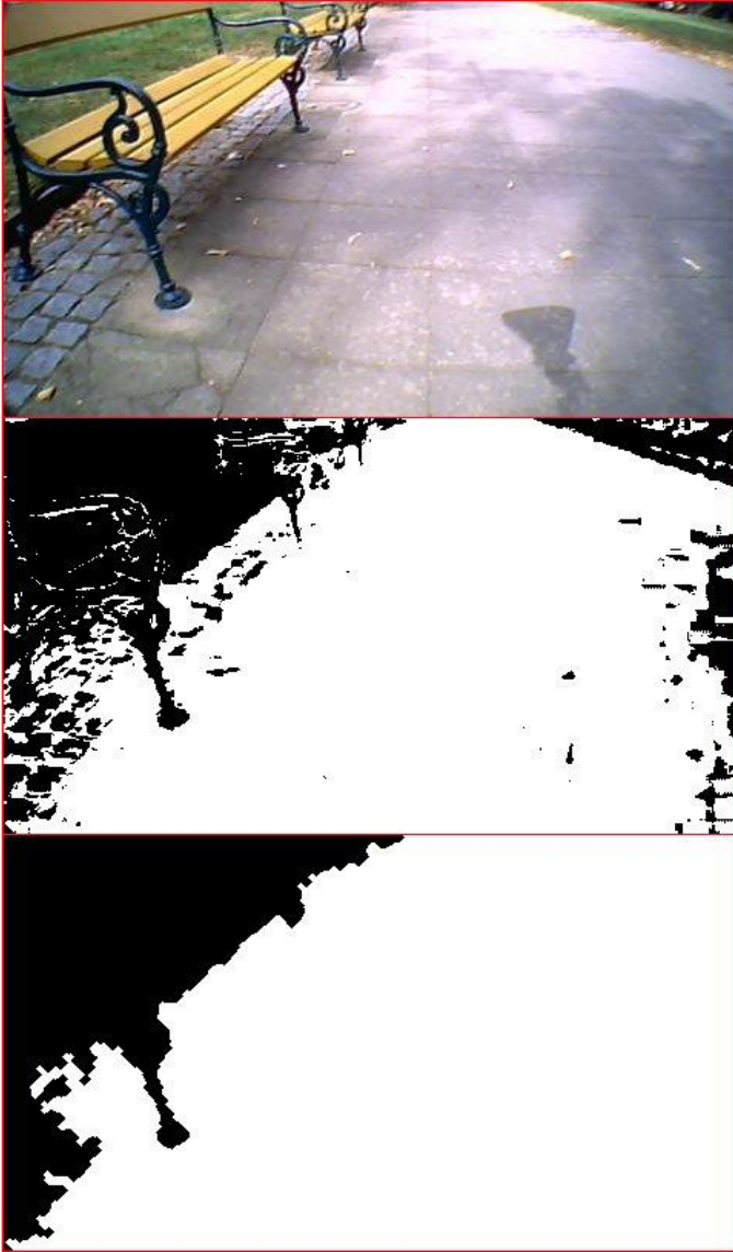
Figure 2. Example of thresholding segmentation and postprocessing. Image was converted to c1c2c3 color space and segmented by thresholding technique. Reference point was obtained from trapezoid region in front of a robot and threshold value is 20. After that, combination of postprocessing methods was applied.
