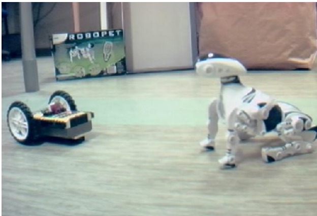
Figure 2. Controlling RoboPet from RCX using IR signals.
