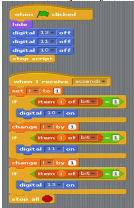
Fig. 2 The S4A code sequence for switching off & on “bits” on Arduino
