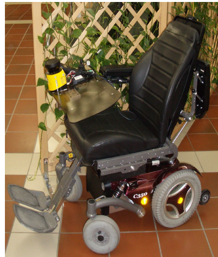
Fig. 1 A Permobil Corpus C350 power wheelchair, from Permobil AB, equipped with a laser range finder (on wheelchair table), a rate gyro, and an USB interface to access the control system.
