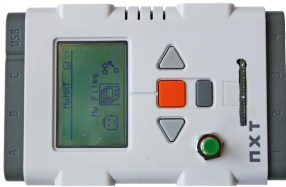
Figure 2 NXT frontside with 1.27" female connector and reset button
