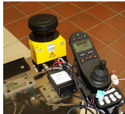
Fig. 2 A laser range finder, mounted on the wheelchair table, was used for perception and detection of obstacles. A rate gyro, to the right of the hand control unit, was to calculate the heading of the power wheelchair
