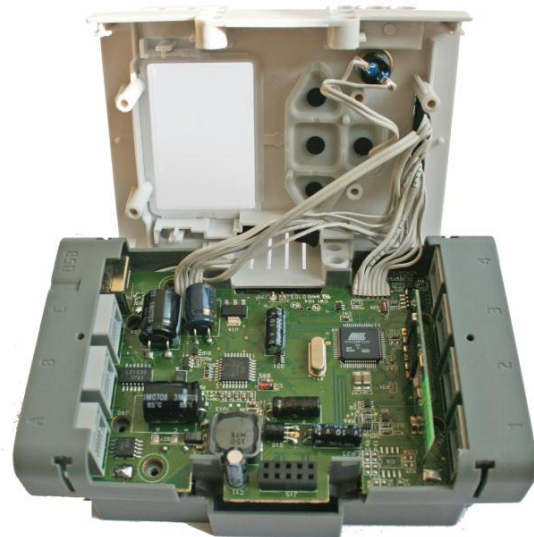
Figure 1: NXT with JTAG modification
