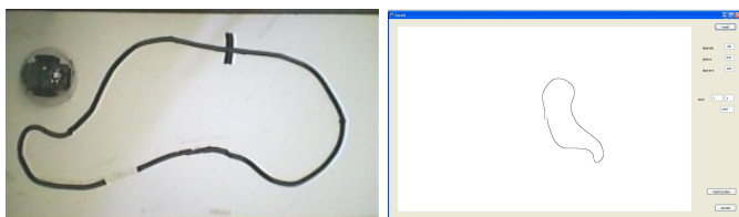
Fig. 5. A simple line track to be mapped by a robot (above) and a resulting map reconstructed from odometry by an application written in Delphi (below), E.Rapcik, R.Stupka.
