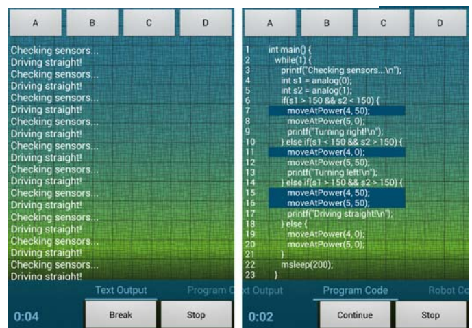
Fig. 2. Two screenshots (cropped) from a debug session. Left: Standard output. Right: Setting breakpoints in the source code while the program is suspended.
