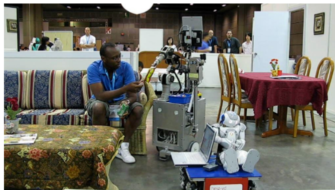
Fig. 8, Our group of robots, RG-Y, including here RH-Y, in background, and OP-Y in foreground, the latter ensuring robust navigation for a humanoid (re. Nao, of Aldebaran Robotics), also integrated, as a mediator, between human and machines, in our applications (re. text) (picture from an HEIG-VD video made during official, international Robocup@Home competition)
